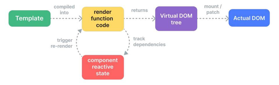
Vue templates containing reactive objects go through a series of steps to result in the render functions that ultimately output the Virtual Node which is used by the Patch Process to create the actual DOM
